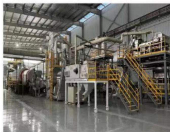
全自动带电破碎锂电池电芯回收生产线 auto charged crushing lithium battery recycling machine
